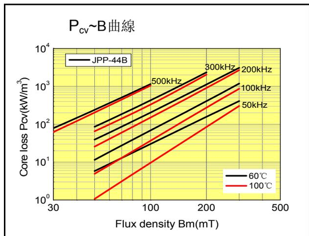
Test core: OD=25mm TH=8mm ID=15mm
